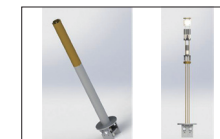
External (left) and internal views of 2-Channel NMR Probe (right)
