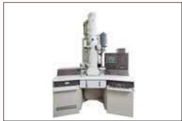
고분해능 투과전자현미경 High-resolution transmission electron microscope(HR-TEM)
