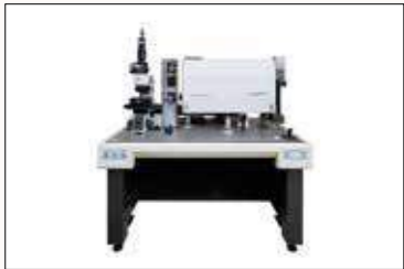
마이크로라만분광기 Micro Raman spectroscopy system (Micro-Raman)
