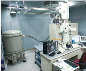
• Field Emission Transmission Electron Microscope(200KV)
